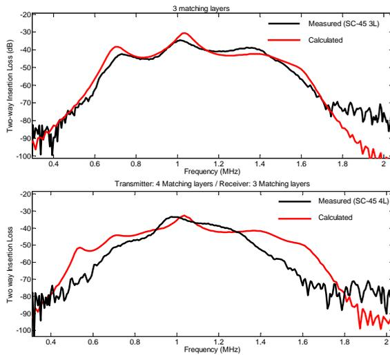
Figure 6. Measured and calculated frequency bands of the SC transducer with two different matching layers configurations in pitch-catch configuration.
