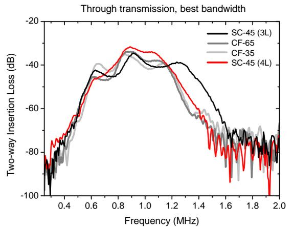
Figure 4. Two-way Insertion Loss. Optimum bandwidth configuration.
