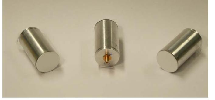
Figure 2. Prototype transducers for efficient air-coupled operation. Transducer aperture: 20 mm
