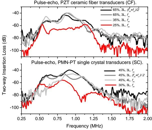
Figure 3. Two-way Insertion Loss of the air-coupled transducers made with the 1-3 connectivity in Table III.
