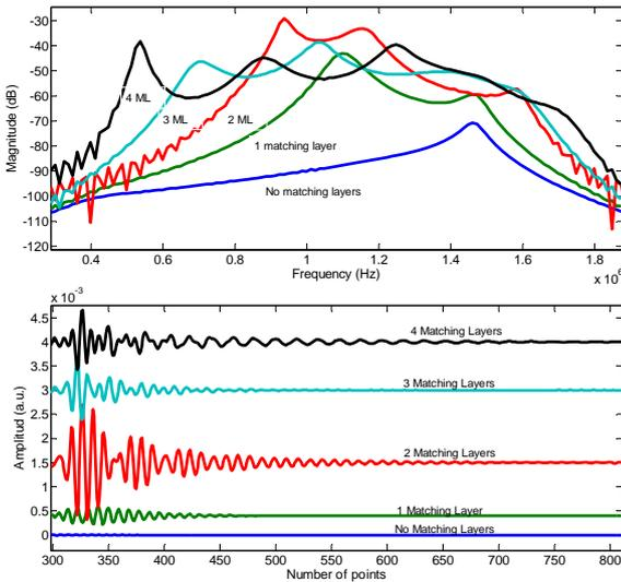
Figure 1. Calculated frequency band and signal in the time domain for pitch-catch operation. Separation between transmitter and receiver 10 mm.
