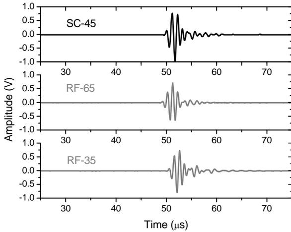
Figure 5. Impulse response in through transmission mode. Pulsar: 5078 Panametrics; pulse amplitude: 400 V; gain: 0 dB; separation: 17 mm.
