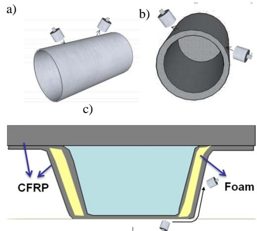
Figure 5. Schematic representation of the experimental set up for the study of axial Lamb wave propagation in a steel pipe, circumferential Lamb wave in a pressure vessel and Lamb wave propagation along in the curved section of a beam.
