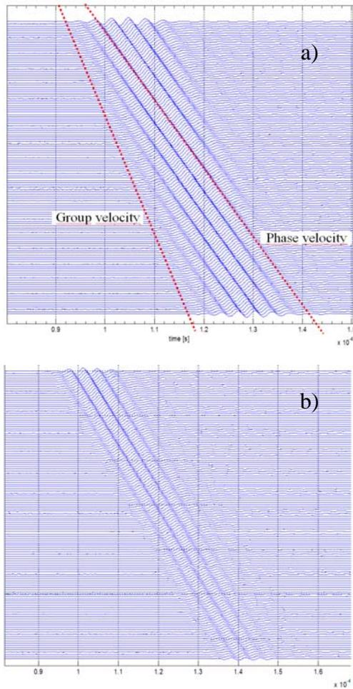
Figure 2. Waterfall representation of the a-scans of the Lamb wave received when the distance between transducers is increased (total scan distance: 130 mm, steps: 0.5 mm and 0.25 MHz. a) Aluminium, b) Cured CFRP.
