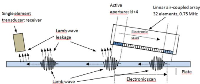
Figure 3. Schematic view of the experimental set-up to using one air-coupled linear array (transmitter) and one single element (receiver).
