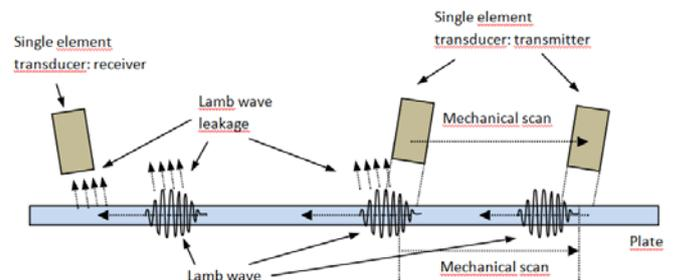
Figure 1. Schematic view of the experimental set-up to visualize Lamb wave propagation in plates using two single element air-coupled transducers and mechanical scan along the propagation direction.
