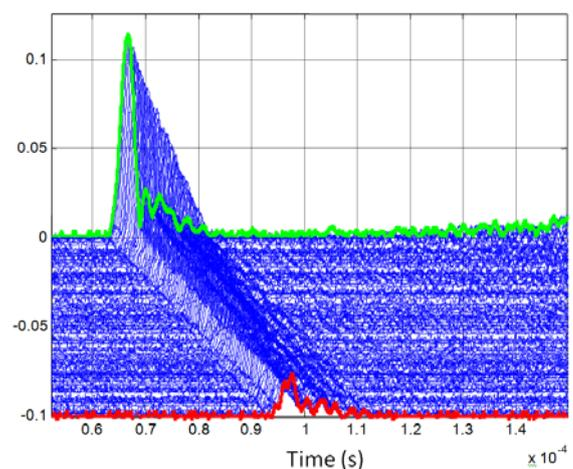
Figure 8. Waterfall representation of the Hilbert transform of the Lamb wave as the distance between transducers is increased. CFRP plate 0.65 MHz.
