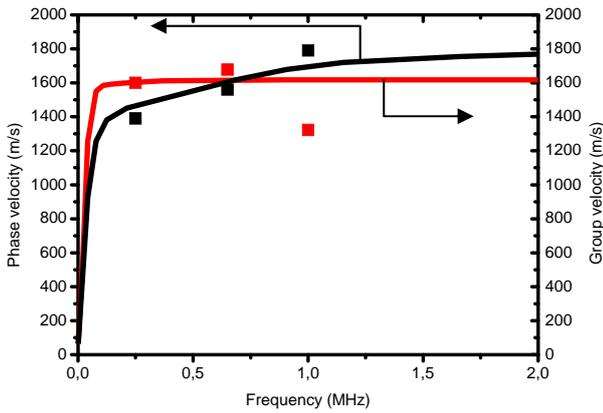
Figure 9. Phase (black) and group (red)  $A_0$  Lamb wave velocities in the 2.1 mm thick CFRP plate. Solid line: theoretical relation dispersions, Dots: experimental data.
