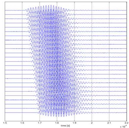
Figure 4. Waterfall representation of the a-scans of the Lamb wave received in the receiver transducer when the distance travelled by the Lamb wave is increased. Aluminum plate and linear array and single element transducers.
