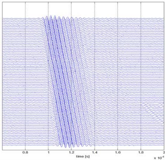
Figure 6. Waterfall representation of the a-scans of the Lamb wave received in the receiver transducer when the distance travelled by the Lamb wave is increased. Steel pipe and 0.25 MHz. Difference between phase and group velocity is clearly appreciated.
