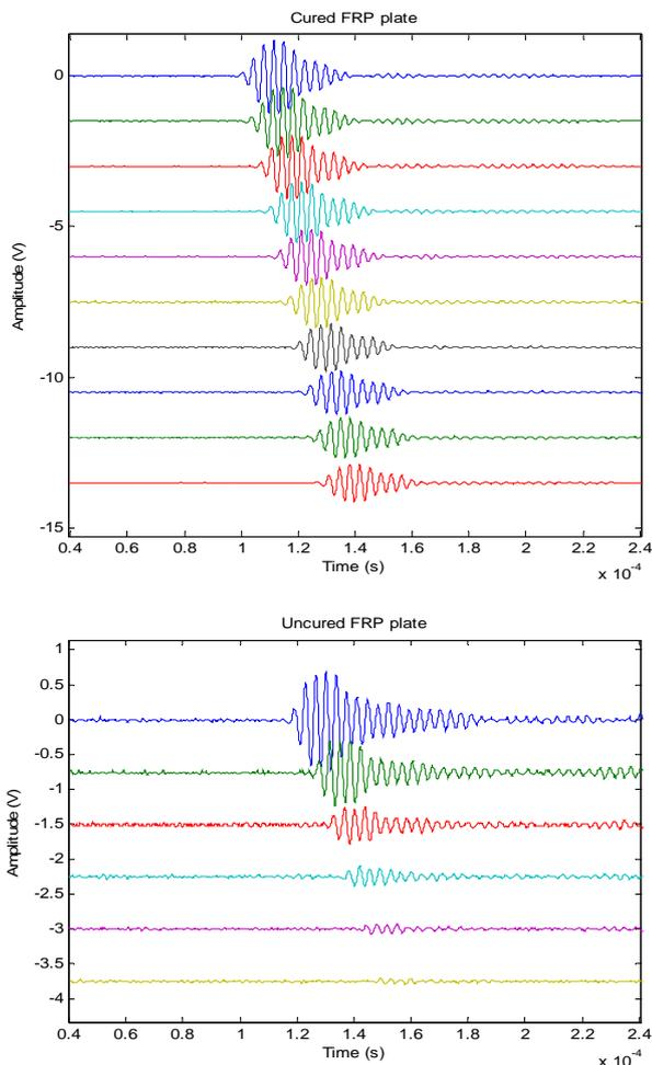
Figure 7. A-scans of the Lamb wave received in the receiver transducer when the distance travelled by the Lamb wave is increased in steps of 5 mm.
