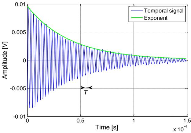
Fig. 5. Temporal signal and the approximation by an exponential function.
