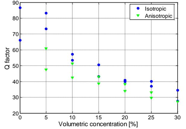
Fig. 6. Quality factor obtained by the temporal signal in function of the volumetric concentration.
