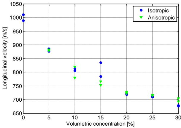
Fig. 8. Longitudinal velocity from the spectrum approach in function of the particle volume fraction.
