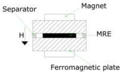
Fig. 1. Sketch of the anisotropic pre-structure device.
