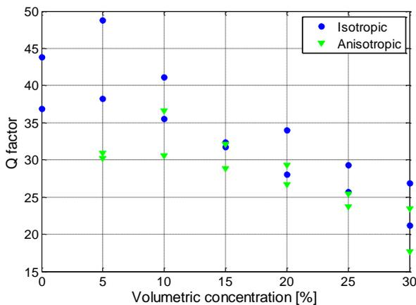
Fig. 9. Quality factor obtained from the spectrum approach at the resonance frequency in function of the volumetric concentration.
