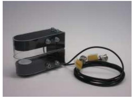
Fig. 2. Picture of the transmitter-receiver pair of transducers embedded in the U-shaped holder for air-coupled through transmission measurements. The slot between transmitter and receiver is used to place the samples.
