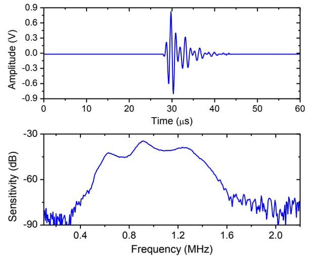
Fig. 3. Up: transmitted signal from transmitter to receiver in the time domain without any sample between them. Down: sensitivity vs frequency
