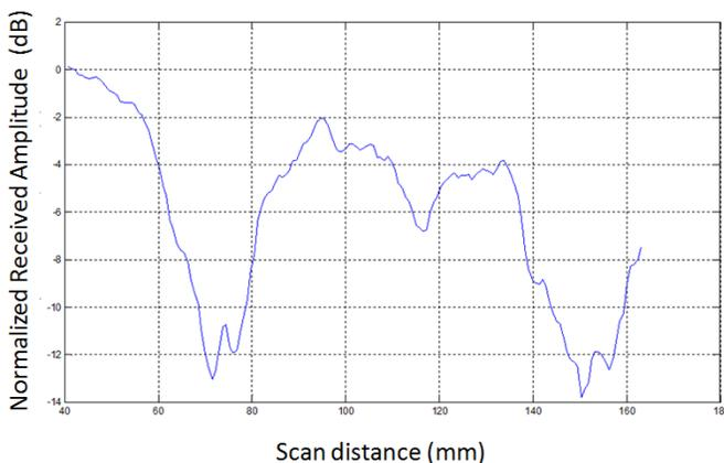
Fig. 7. Linear scan along two Teflon insertions, laminate with 24 layers measured after a long compaction.
