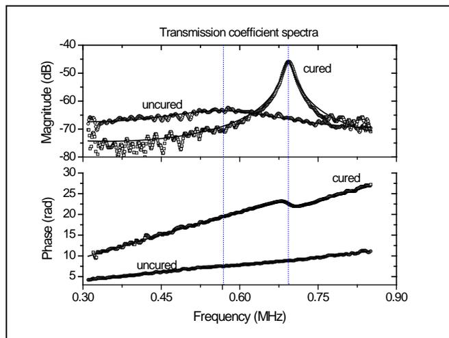
Fig. 2. Measured and calculated magnitude and phase spectra of the transmission coefficient for two FRPC plates, cured (2mm thick) and uncured (1 mm thick).
