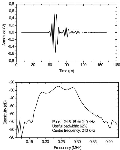
Fig. 4. Measured impulse response and sensitivity of the 0.25 MHz air-coupled transducers employed for the tests.
