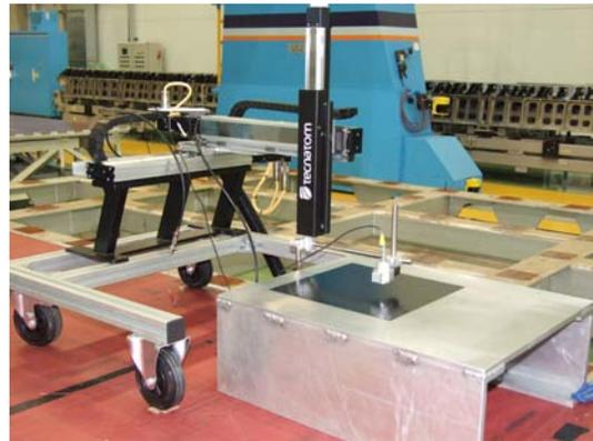
Fig. 5. Picture of the aluminum mold with the CFRP, the transducers and the scanning system.
