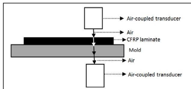
Fig. 1. Proposed configuration for the non-contact inspection of lay-up laminate of CFRP composite on the fabrication mold using a through transmission technique and air-coupled piezoelectric transducers.
