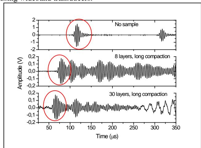
Fig. 6. Transmitted signal from Tx-transducer to Rx-transducer for three cases: Up: no sample between Tx and Rx. Middle: CFRP laminate (8 layers) and 13 mm aluminum mold. Bottom: CFRP laminate (30 layers) and 13 mm aluminum mold.
