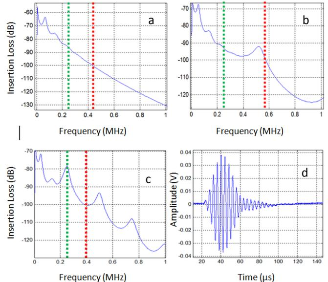
Fig. 3. Calculated spectra of the Insertion loss of the FRCP laminate and the aluminum mold for three different mold thicknesses (a: 2 mm; b: 6 mm; c: 13 mm). Green line indicated the location of the 0.25 MHz frequency and the red line indicates the maximum inspection frequency for the -100 dB limit. 3. d: simulated transmitted pulse for the 13 mm mold using a pair of 0.25 MHz air-coupled transducers.
