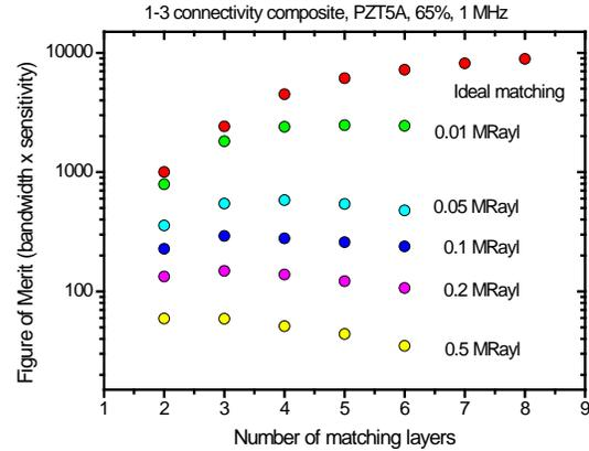
Figure 3. Variation in  $fom$  with the number of matching layers for a given value of  $Z_n$
