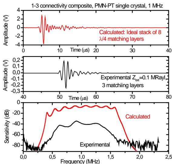
Figure 6. Theoretically calculated response (Tx-Rx) of the air-coupled transducer with an ideal stack of  $\lambda/4$  impedance matching layers and measured response (Tx-Rx) of the prototype built with the novel proposed materials and design procedure.
