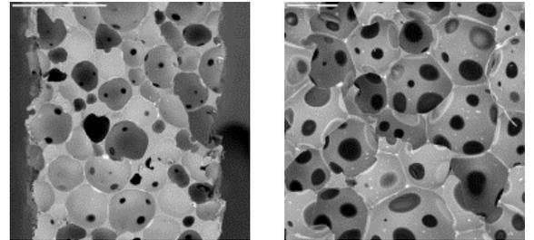
Figure 5. SEM images of cross-sections of two of the cellular rigid solids proposed as low  $Z$  and high  $v$  matching layers
