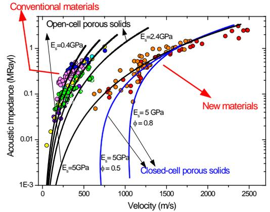
Figure 4. Experimental (dots: green: polymeric membranes, blue: paper, yellow: silica aerogels, pink: vegetal tissues, marine: flexible foams, red and orange: new rigid semiclosed-cell polymeric foms) acoustic impedance versus ultrasound velocity and theoretical values according to Eqs. (4) and (5) for several values of the Young modulus of the solid and for two different porous structures: open-cell and closed cell.
