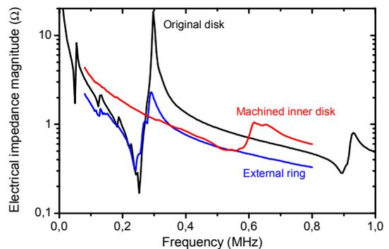
Fig. 2. Electrical impedance vs. frequency of the original 1-3 connectivity piezocomposite disk, and the machined external ring and inner disk.
