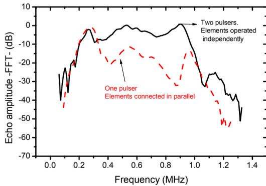
Fig. 7. Normalized response in pulse-echo, water immersion of the whole array under two different excitation conditions: magnitude of the FFT of the echo reflected by an aluminium block.
