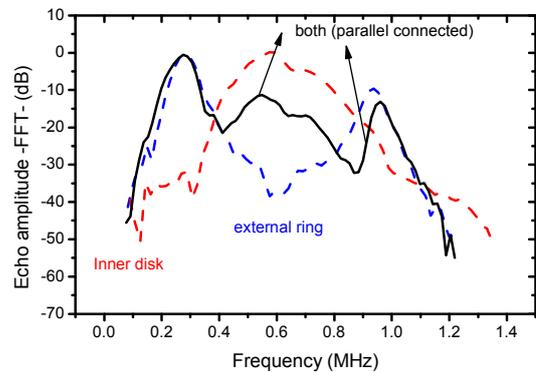
Fig. 6. Normalized response in pulse-echo, water immersion of the individual elements and the whole array: magnitude of the FFT of the echo reflected by an aluminium block.
