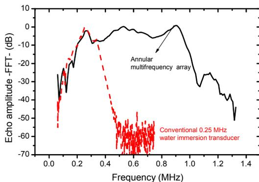
Fig. 8. Normalized response in pulse-echo, water immersion of the whole array and of a conventional 0.25 MHz centre frequency water immersion transducer.
