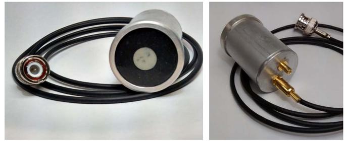
Fig. 5. Picture of front (right) and back face of the transducer prototype with the BNC terminated cable.
