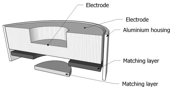
Fig. 4. Schematic view of the array cross-section structure: mechanized disk (central disk and external ring), matching layers and aluminum housing.
