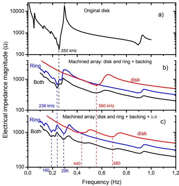
Fig. 3. Magnitude of the electrical impedance (magnitude) vs. frequency for the original disk (a), the annular array with the backing (b) and the annular array with the backing and the matching layers.
