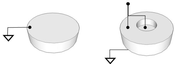
Fig. 1. Schematic representation of the original 0.25 MHz resonant frequency piezocomposite disk (left), and the mechanized two elements annular array: external ring with resonant frequency at 0.25 MHz and internal disk with resonant frequency at 0.55 MHz.
