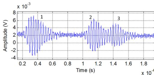
Fig. 3 Received Lamb wave in a 1.5 mm thick aluminum plate
