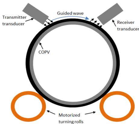
Fig. 3. Setup for the pitch-catch configuration mode.
