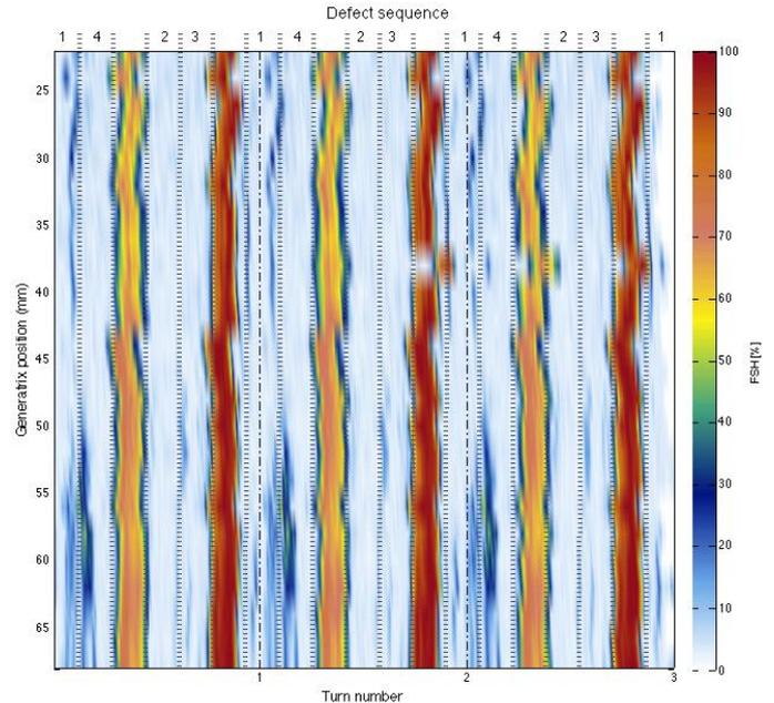
Fig. 4. C-Scan image obtained using the configuration mode 1.
