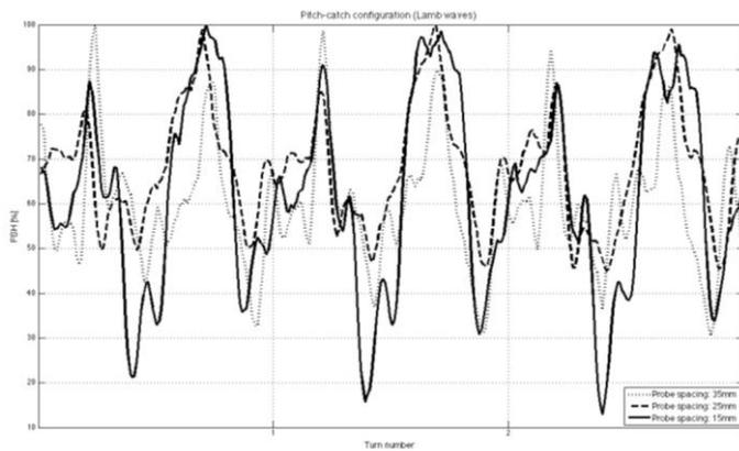
Fig. 6. Test adjusting the sound path on the cylinder wall at 15 mm, 25 mm, and 35 mm. Each response corresponds to three turns of the cylinder, acquired at 36 mm from the edge. The defects sequence is 1-4-2-3.
