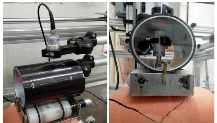
Fig. 2. Arrangement for scanning the sample under test in through-transmission mode. At the top is the emitter transducer, inside the receiver.
