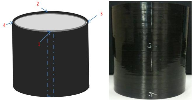
Fig. 1. Diagram of insert locations and picture of the test tube with aluminum liner overwrapped with carbon fibre used in the experimentation.
