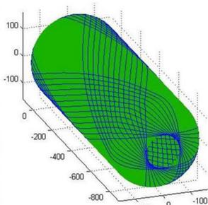
Example of filament winding process of a composite overwrapped pressure vessel.
