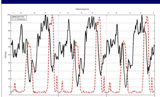
Comparison between data obtained using guided waves and through-transmission mode. Signals were taken at 36 mm from the cylinder edge.
