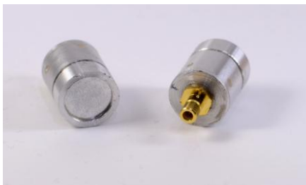
Fig. 1. Picture of the two 10 mm diameter prototypes of water immersion transducers using FF film (left: front face, right: rear face with SMB connector).
