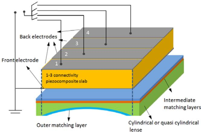
Fig. 2. Scheme of the linear array transducer: elements distribution and lens orientation
