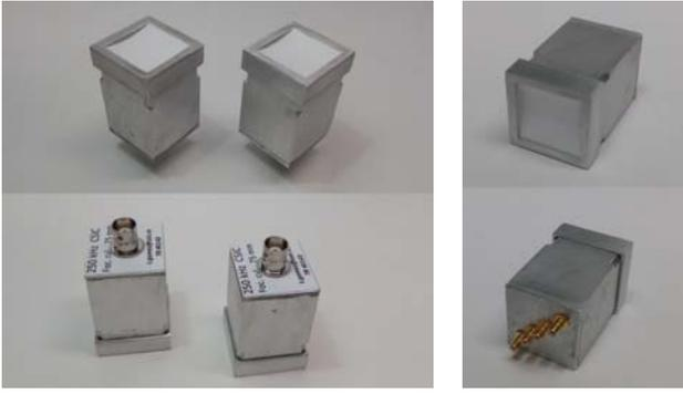
Fig. 1. Picture of the 250 kHz cylindrically focused air-coupled transducers. Left: Monolithic transducers. Right: 4-elements linear array.
