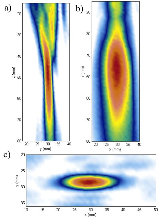
Fig. 6. Measured acoustic field of the element 3 of the array transducer in planes (a) YZ (b) XZ and (c) XY at  $Z = 47 \text{ mm}$ .
