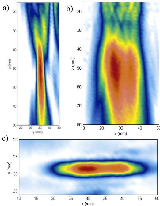
Fig. 5. Measured acoustic field of the monolithic transducer in planes (a) YZ (b) XZ and (c) XY at  $Z = 49 \text{ mm}$ .
