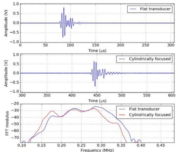
Fig. 4. Magnitude of the FFT of the received signal in through transmission of flat (blue), cylindrically focused (red) transducers.
