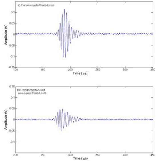
Fig. 9. Generation and detection of  $A_0$  mode in Al plate.
