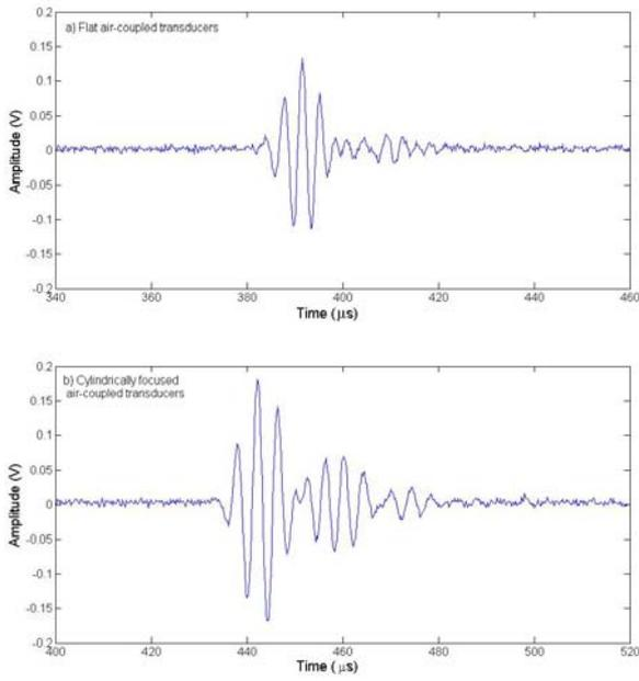
Fig. 7. Through transmission through a cylindrical pipe wall. 7.a. Flat air-coupled transducers. 7.b. Cylindrically focused air-coupled transducers.
