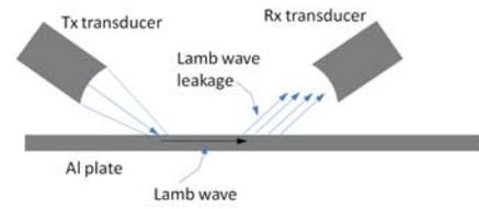
Fig. 8. Schematic representation of the use of cylindrically focused air-coupled transducer to generat and receive Lamb waves in plates.
